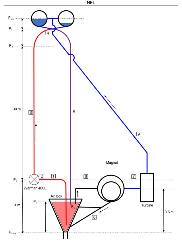
Figure 1 Overview and schematic of the ECS.
